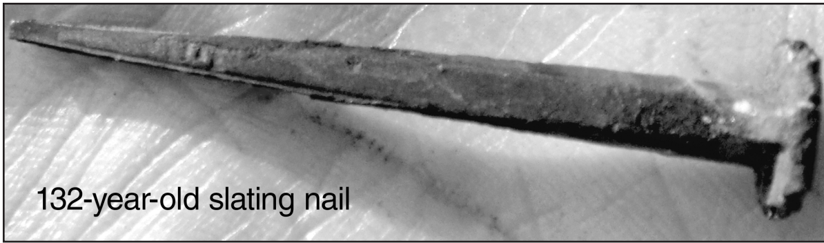
Figure 9 – Just because the roof is old doesn't mean the nails have gone bad. This slating nail was pulled off a Buckingham slate roof on an 1879 church in Virginia in 2011 (Photo by Joseph Jenkins).
