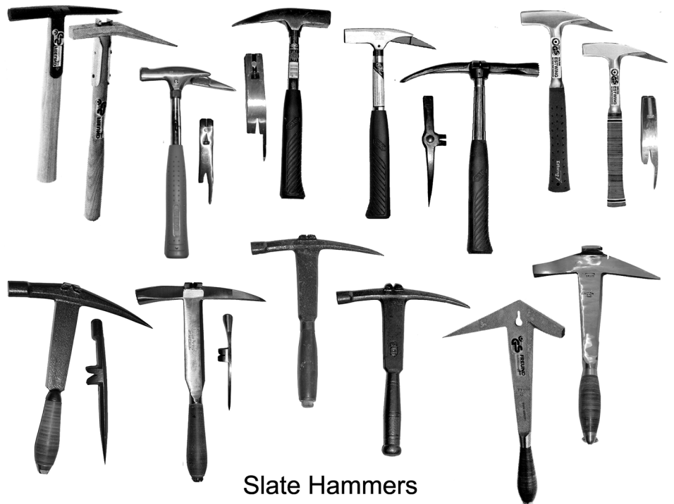
Figure 12 – Slate hammers come in a variety of shapes and styles. They all have a pointed pick end that is used to punch nail holes in slates.
